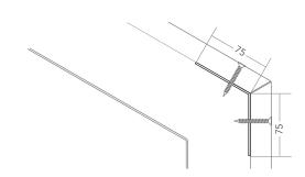
The Angle Profile is used to connect two different planes of cladding material. It serves to provide a fixing point for the edge of the cladding material and hold the two edges in relation to each other. This is particularly useful for connecting timber cladding at a change of pitch or plane as over time, the timber can warp and twist. As an option, it can be supplied with a matt black finish where there is a requirement for it not to be visible between open cladding joints.
