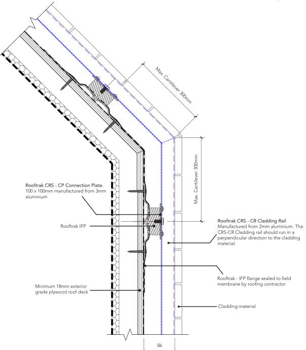
The versatile ROOFTRAK® IFP can be used for a range of cladding applications and solar panel arrays on pitched and flat roofs.
