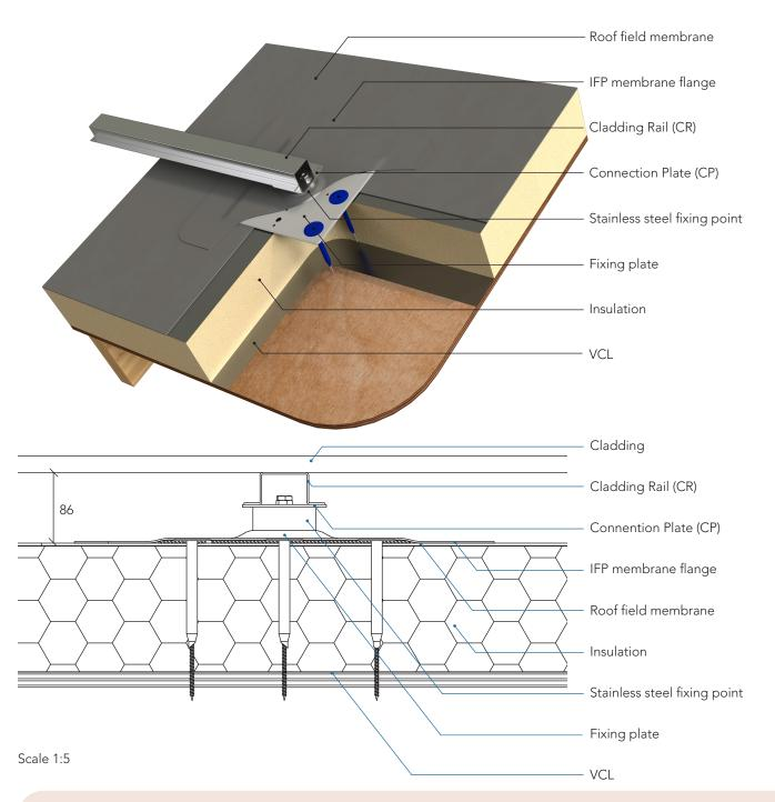
The IFP-300 is designed for use on warm roof constructions and where the roofing membrane is laid on directly on insulation including composite panel systems. It comprises a 300mm x 300mm fixing plate and an anchor point with two M10 x 20 blind threads. To weather the fixing plate the IFP-300 is factory fitted with an appropriate flange material to enable it to be weathered or sealed to the main roof area. These must be installed with the fixing holes in line with the Cladding Rail direction.
