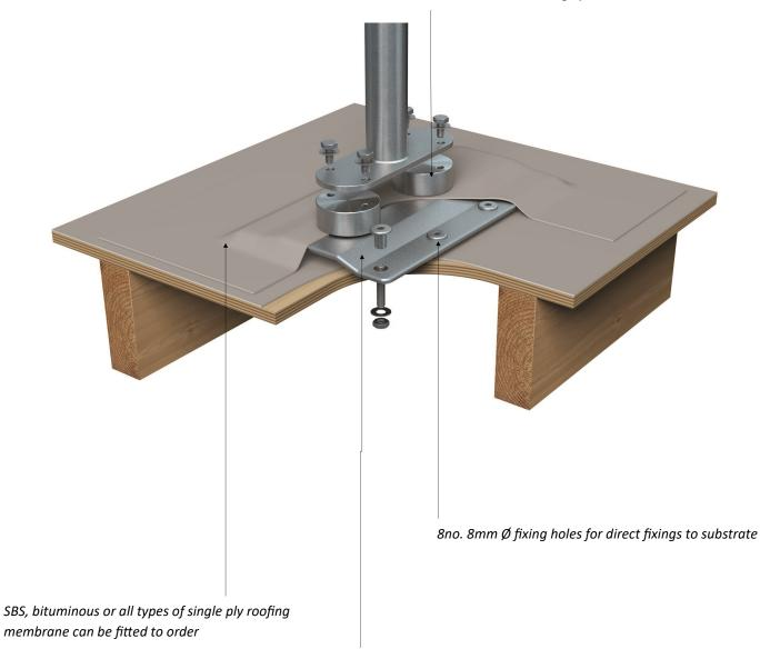
2no stainless steel fixing point 33mm high x 76mm Ø with 2no M10 threaded anchorage points
