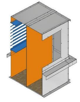
**17. Either** make duct connections to the ply base before installation
