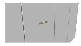
**Step 1** Cut a letterbox hole as small as possible. Make good cut edges with touch up paint.
